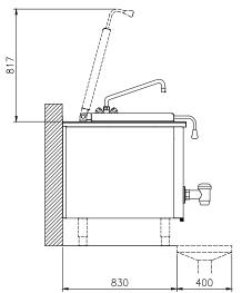
CWII Cold Water inlet 1 (cleaning) Electrical inlet (power)
